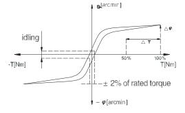
**Return gap JT [Arcmin]:** The maximum deviation of the output shaft of the speed reducer and the input angle. When measuring the gear input end is fixed, and then use the torque meter load certain torque at the output (2%T2B), to overcome the friction force in the speed reducer
